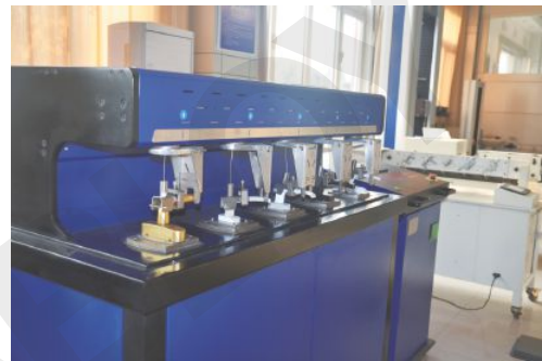
Handle Life-Cycle Testing Machine
