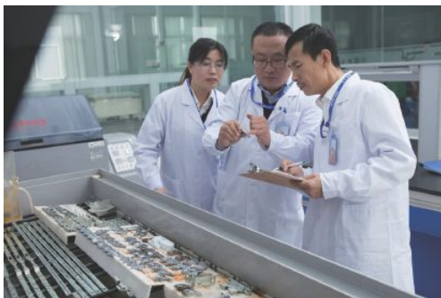
Salty Spray Testing Instrument
